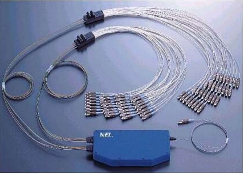
100 GHz Spacing, 40 channels, Gaussian
