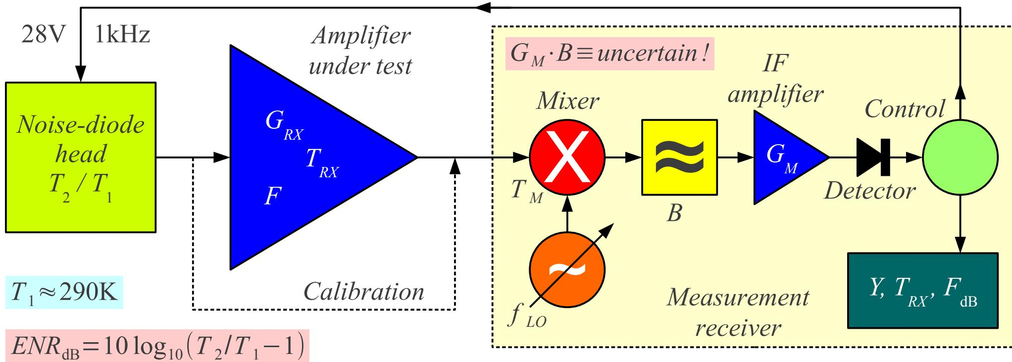
Two measurements without calibration
