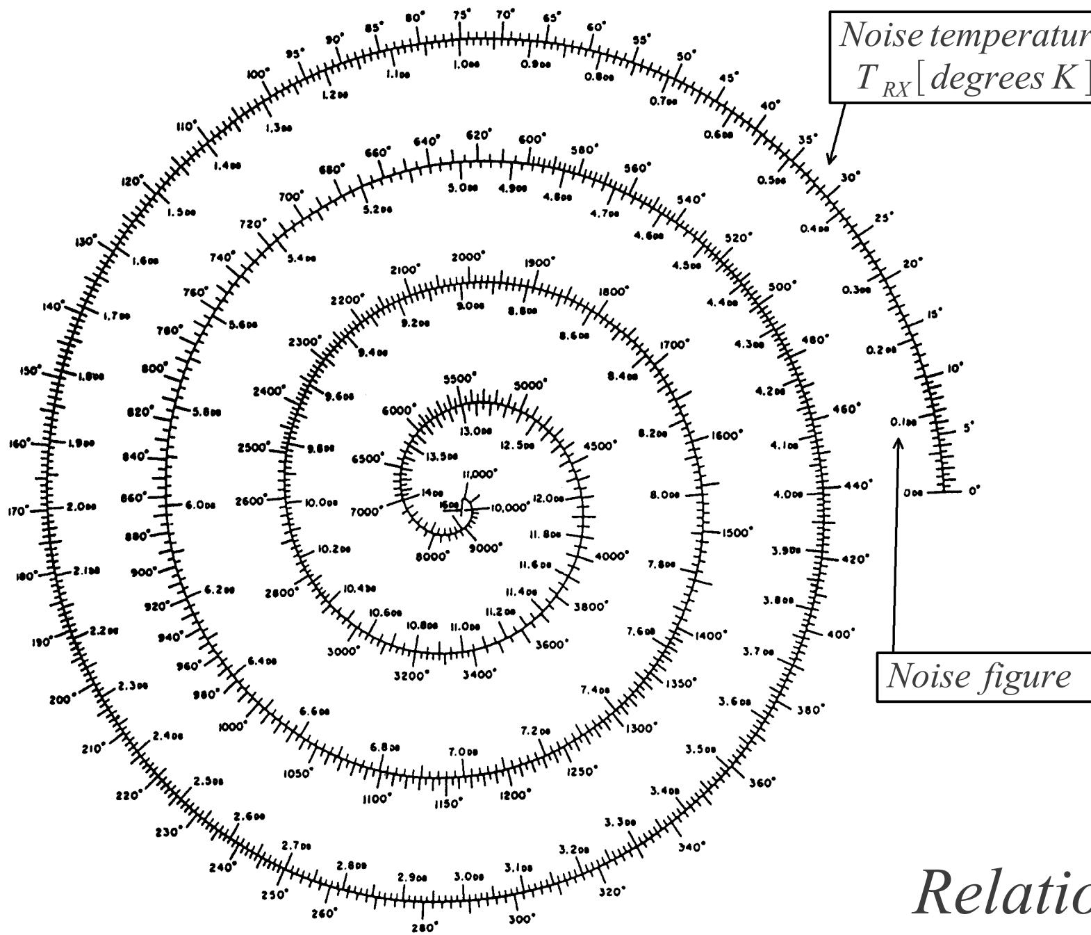
$$F_{\text{dB}} = 10 \log_{10} \left( 1 + \frac{T_{\text{RX}}}{290\text{K}} \right)$$
