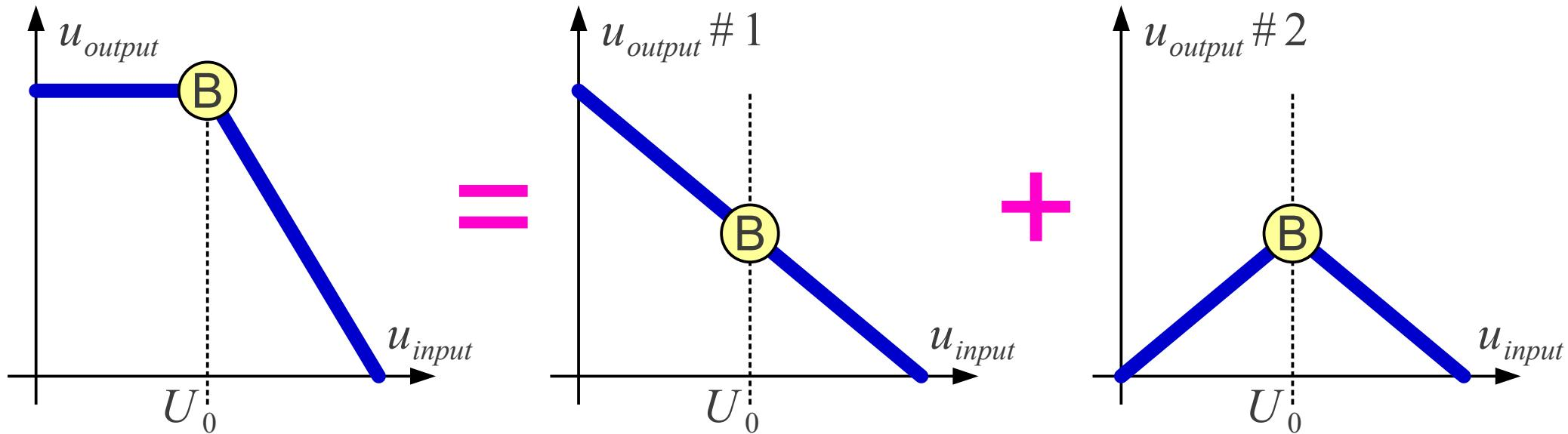
$$u_{output} \# 1 = \alpha_0' + \alpha_1 \cdot (u_{input} - U_0) \equiv \text{rectilinear}$$
