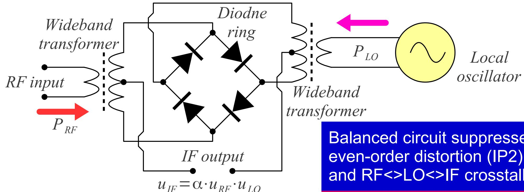
Balanced circuit suppresses even-order distortion (IP2) and RF<>LO<>IF crosstalk
