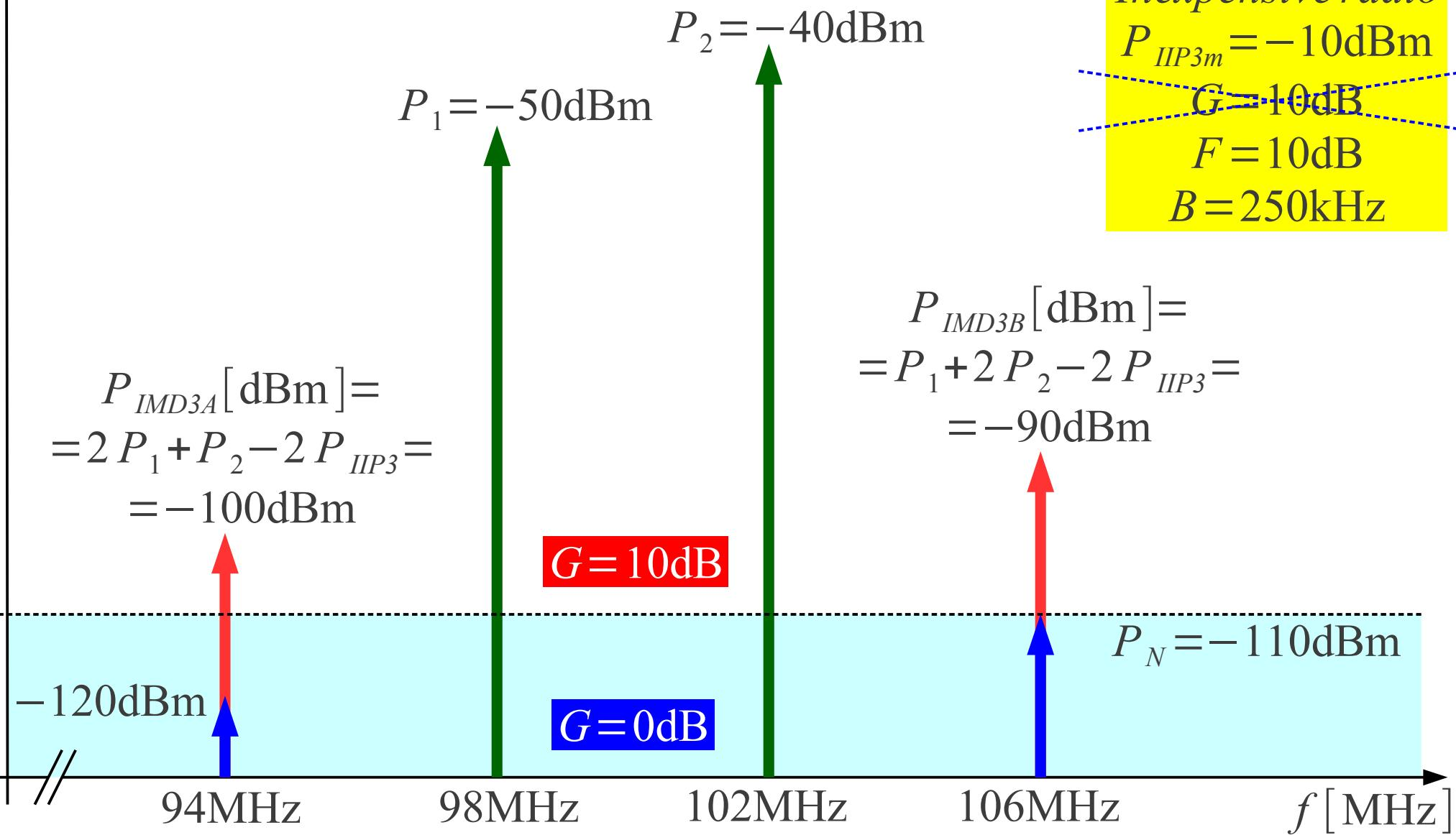
$$P_N = 10 \log B + 10 \log k_B T_0 + F_{\text{dB}} \approx 54\text{dB.Hz} - 174\text{dBm/Hz} + 10\text{dB} = -110\text{dBm}$$
