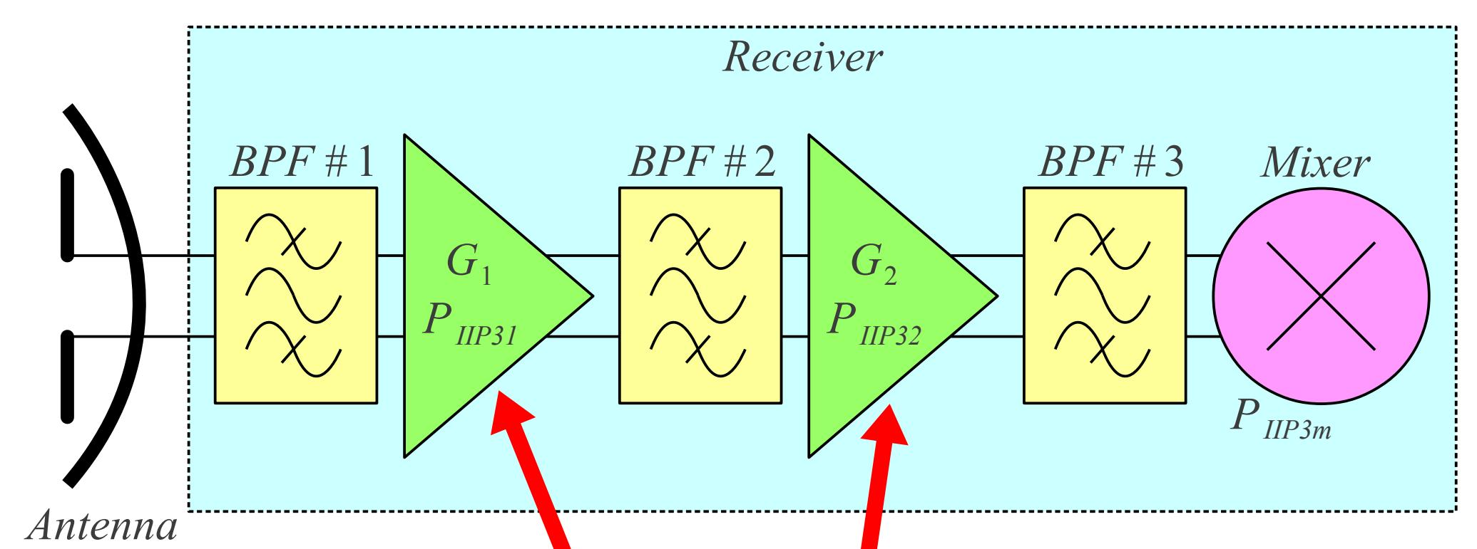
$$P_{IIP3chain} = \frac{1}{\frac{1}{P_{IIP31}} + \frac{G_1}{P_{IIP32}} + \frac{G_1 \cdot G_2}{P_{IIP3m}}}$$
