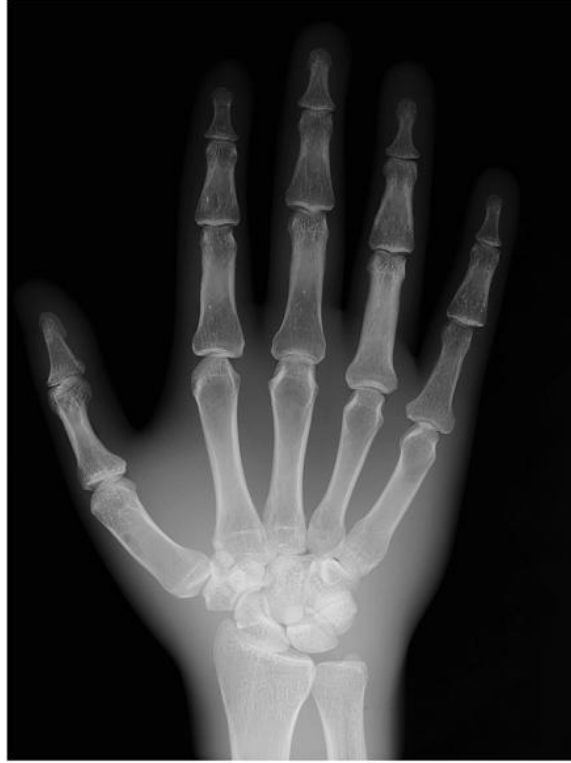
Figure 1.5 An x-ray image of a phantom hand obtained from a direct conversion flat-panel X-ray image detector that uses a stabilized a-Se photoconductor. The AMA has 1,280 \times 1,536 pixels. The image is provided courtesy of Sterling Diagnostic Imaging.
