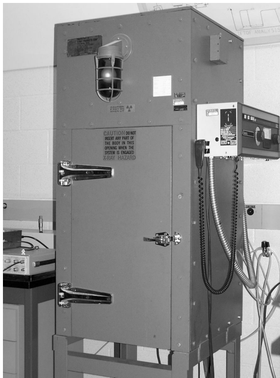
Figure 4.19 This lead cabinet shields the experiment operator from exposure to x-ray radiation. The controls for the x-ray system are mounted on the right hand side of the cabinet. The light above the door indicates that the x-ray system is activated.
