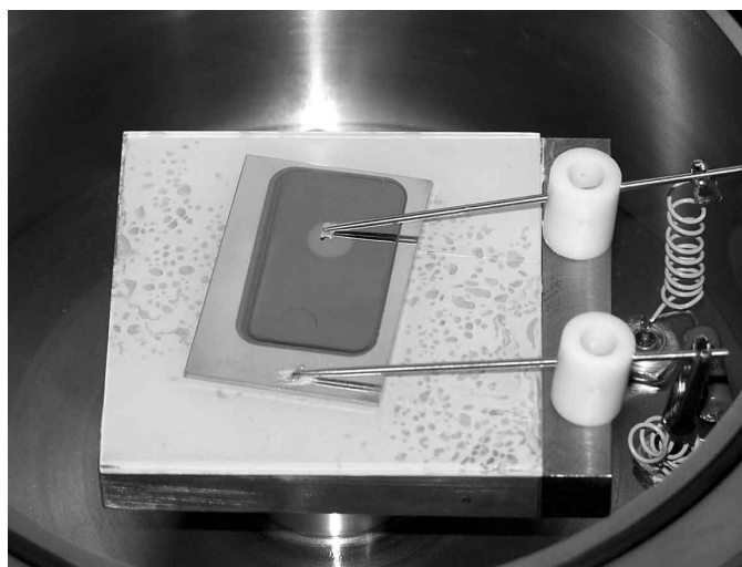
Figure 4.3 The sample loaded in the sample holder ready for TOF and IFTOF transient photoconductivity measurements.
