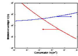
Breakdown voltage and breakdown field versus doping density for an abrupt  $p-n$  junction, 300 K
