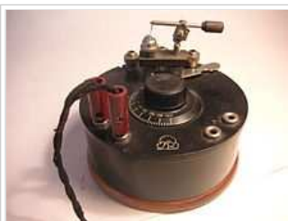
A small portable crystal radio with a cat's whisker detector visible at top
