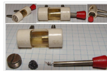
A crystal detector in commercial form from the 1960s
