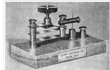
Precision cat's whisker detector using iron pyrite crystal, early-1900s. The crystal is inside the metal capsule under the vertical needle "whisker" ( right ). The leaf springs and thumbscrew allowed fine adjustment of the pressure of the needle on the crystal.
