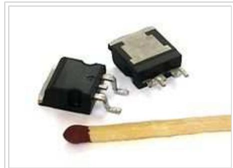
Two power MOSFETs in the surface-mount package D2PAK. Each of these components can sustain a blocking voltage of 120 volts and a continuous current of 30 amperes.
