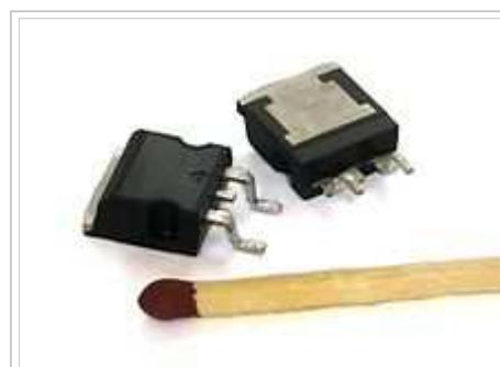
Two power MOSFETs in the surface-mount package D2PAK. Each of these components can sustain a blocking voltage of 120 volts and a continuous current of 30 amperes.
