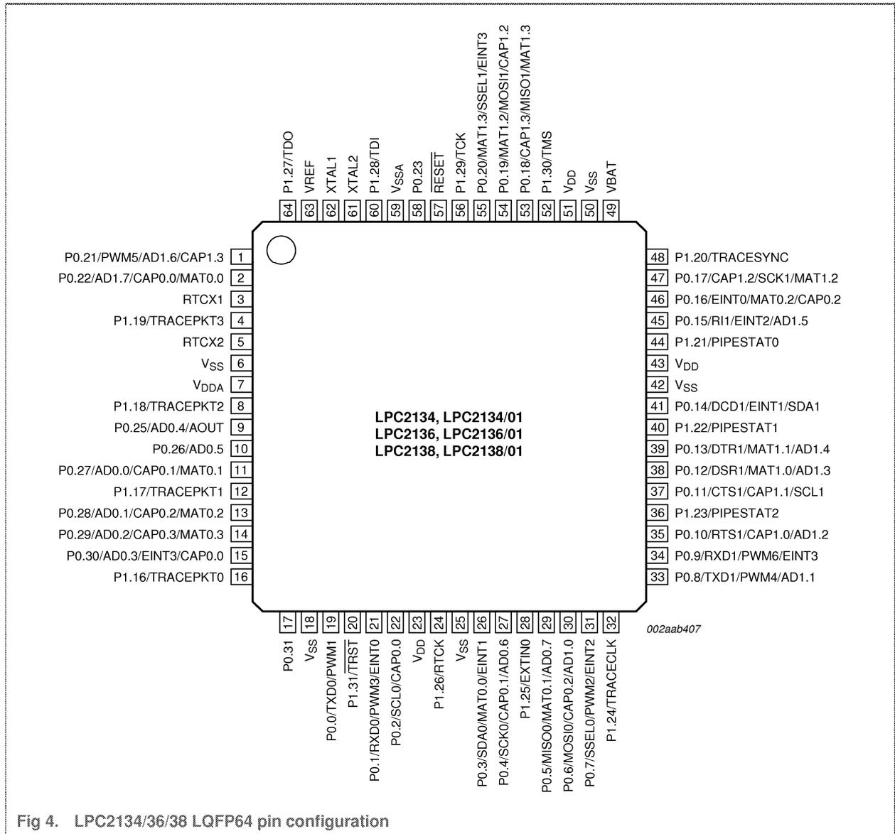
Fig 4. LPC2134/36/38 LQFP64 pin configuration
