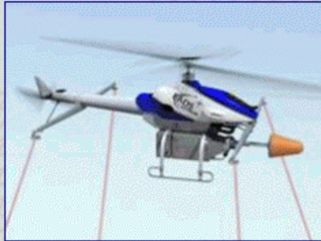
Airborne Near-field Scanner System for Large Scan Contours (Airborne Near-field Test Facility - ANTF)
