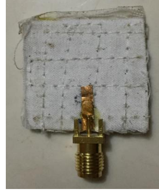
Figure 6: Front and back Side of Prototype Textile antenna with Cotton Substrate)
