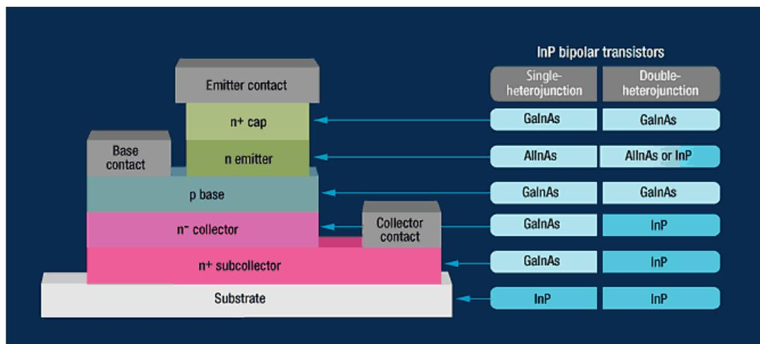
**[2]** Single- and double-heterojunction bipolar transistors (SHBTs and DHBTs, respectively) are made using a combination of materials, but start with an indium phosphide substrate. The ratio of gallium to indium in these transistors is 47:53, and the ratio of aluminum to indium is 48:52.
