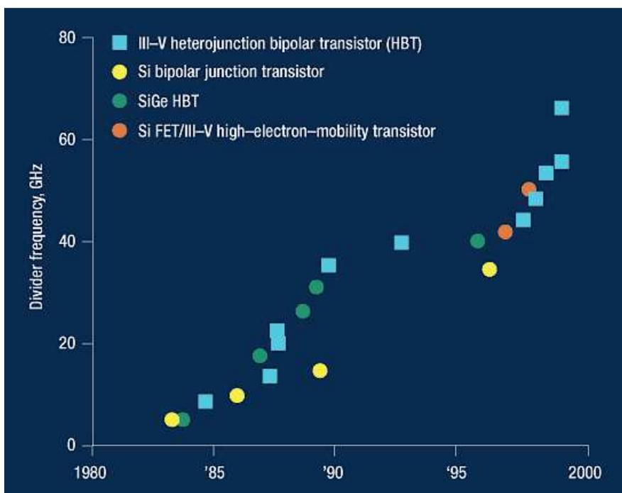
[6] Historically, heterojunction bipolar transistors (HBTs) made using indium phosphide or other III-V materials yielded the fastest static dividers.
