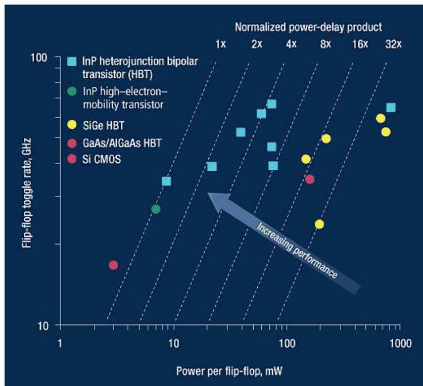
[7] For comparable speeds, indium phosphide flip-flops can consume as little as a tenth of the power of silicon-based devices. Diagonals represent lines of equal power-delay product.
