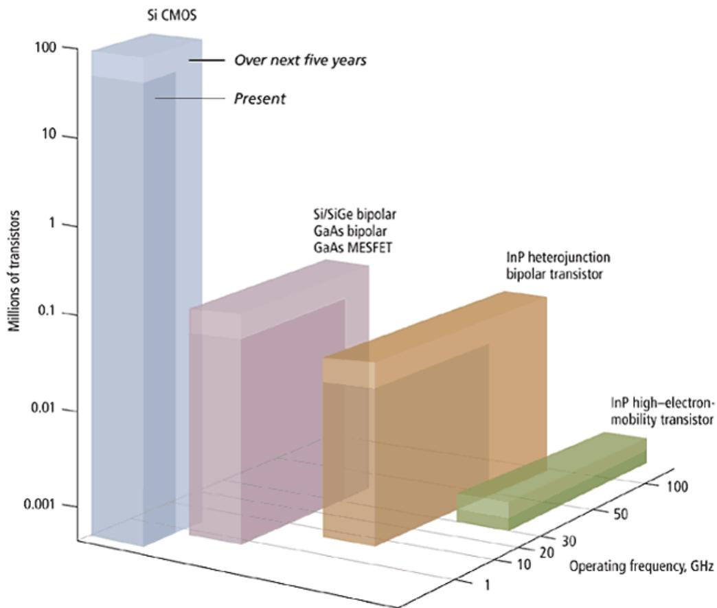
[1] Indium phosphide technology leads all others in operating frequency, but it is not expected to approach the integration scale of silicon chips. Silicon or silicon germanium (Si/SiGe) bipolar transistors and gallium arsenide (GaAs) bipolar transistors and metal semiconductor FETs (MESFETs) have intermediate combinations of speed and level of integration. The current state of the art [dark areas] can expect to improve over the next five years [light areas].
