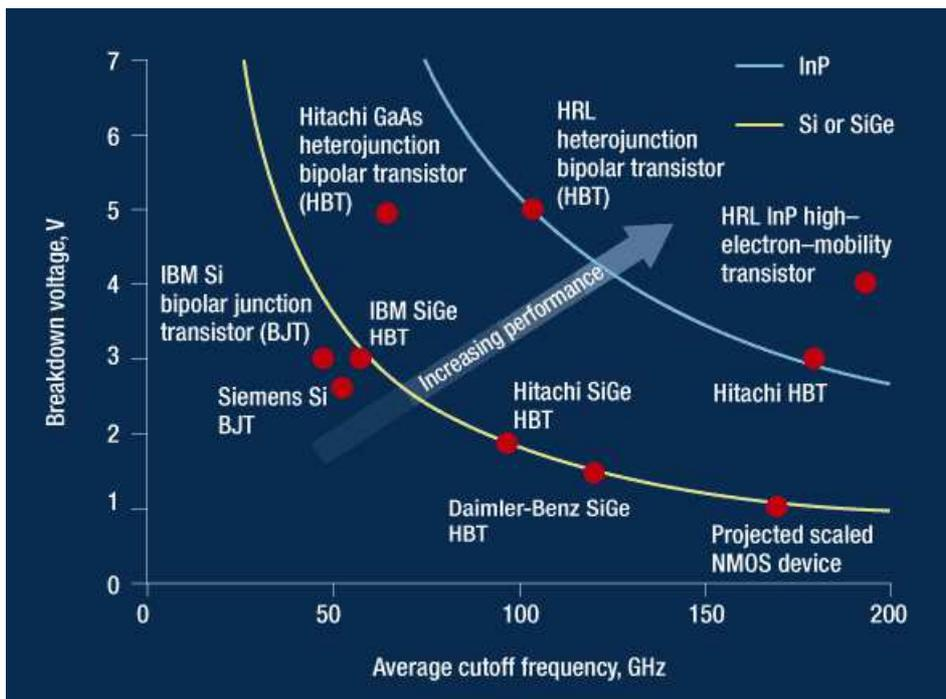
[4] Device breakdown voltage can be traded off for higher average cutoff frequency. For a given breakdown voltage, indium phosphide devices are faster than silicon, silicon germanium, and gallium arsenide devices.
