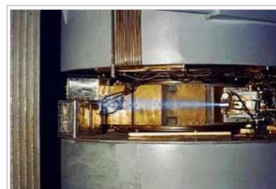
Lawrence's 60-inch cyclotron, circa 1939, showing the beam of accelerated ions (likely protons or deuterons) exiting the machine and ionizing the surrounding air causing a blue glow.
