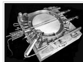
Vacuum chamber of Lawrence 27 in. 1932 cyclotron with cover removed, showing the dees. The 13,000 volt RF accelerating potential at about 27 MHz is applied to the dees by the two feedlines visible at top right. The beam emerges from the dees and strikes the target in the chamber at bottom.
