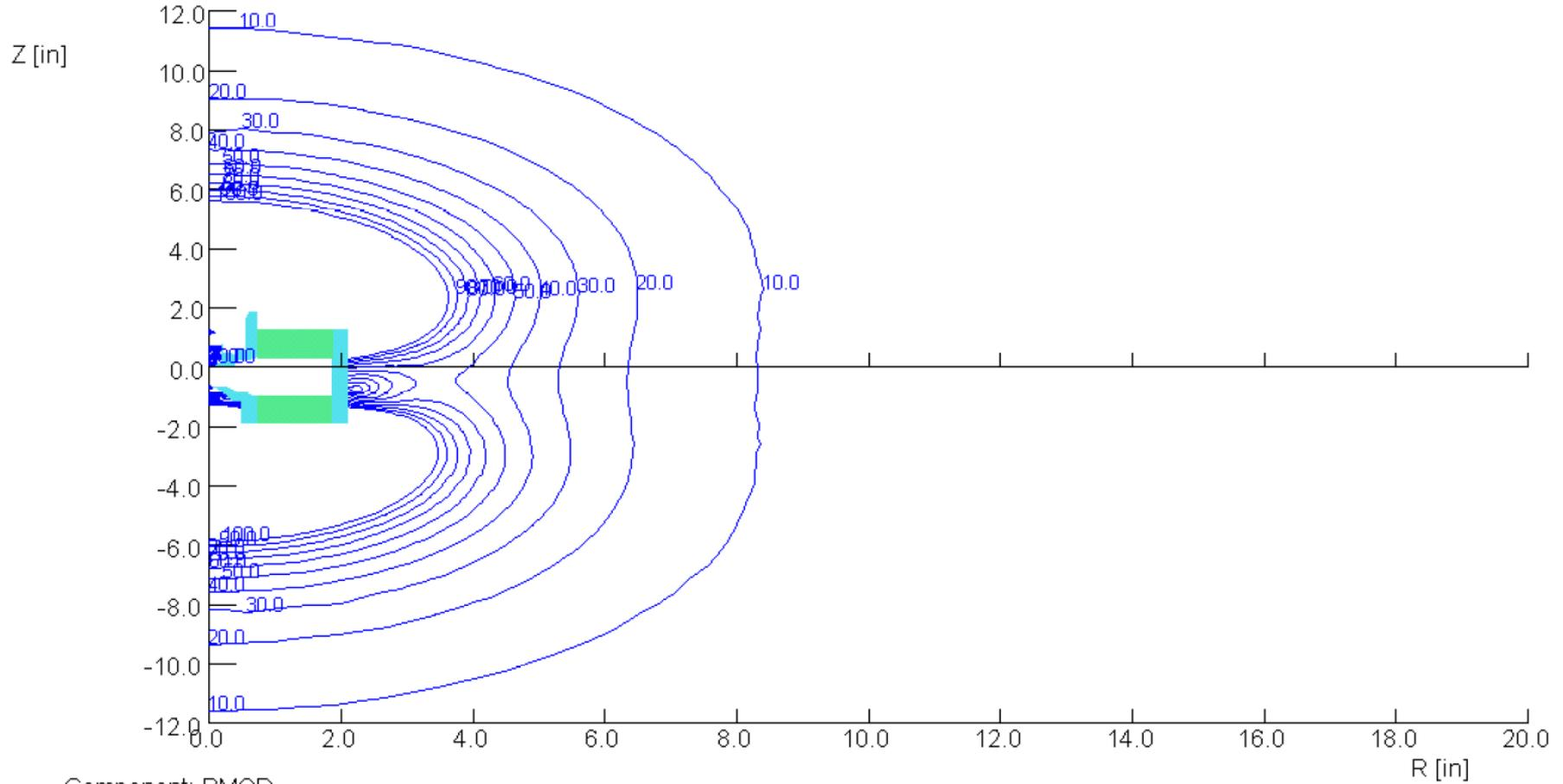
Contours of constant magnetic field (gauss)
