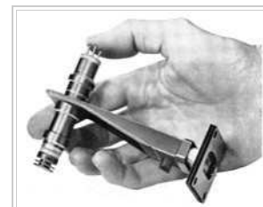
Miniature O-type backward-wave oscillator tube produced by Varian in 1956. It could be voltage-tuned over an 8.2 - 12.4 GHz range and required a supply voltage of 600V.
