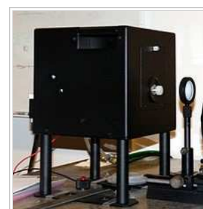
Backward wave oscillator at Stockholm University operating in the Terahertz range
