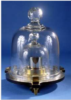
National prototype kilogram K20, one of two prototypes stored at the US National Institute of Standards and Technology in Gaithersburg, Maryland, which serve as primary standards for defining all units of mass and weight in the United States. This is a replica for public display, shown as it is normally stored, under two bell jars.
