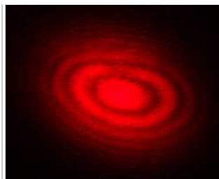
The local gravitational acceleration g is measured with exceptional precision with the help of a laser interferometer. The laser's pattern of interference fringes—the dark and light bands above—blooms at an ever faster rate as a free-falling corner reflector drops inside an absolute gravimeter. The pattern's frequency sweep is timed by an atomic clock.
