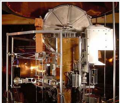
The NIST's watt balance is a project of the U.S. Government to develop an “electronic kilogram.” The vacuum chamber dome, which lowers over the entire apparatus, is visible at top.
