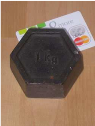
A domestic-quality one-kilogram weight made of cast iron (the credit card is for scale). The shape follows OIML recommendation R52 for cast-iron hexagonal weights [1]
