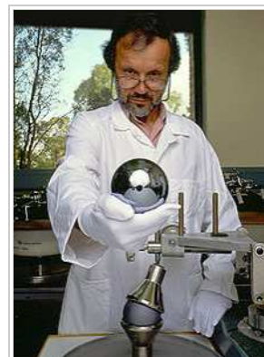
Achim Leistner at the Australian Centre for Precision Optics ( http://www.acpo.csiro.au/ ) (ACPO) is holding a 1 kg, single-crystal silicon sphere for the Avogadro project. These spheres are among the roundest man-made objects in the world. If the best of these spheres were scaled to the size of Earth, its high point—a continent-size area—would rise to a maximum elevation of 2.4 meters above "sea level". [Note 21]
