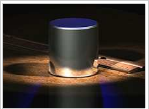
A CGI of the international prototype kilogram (the inch ruler is for scale). The prototype is manufactured from a platinum–iridium alloy and is 39.17 mm in both diameter and height, its edges have a four-angle (22.5°, 45°, 67.5° and 79°) chamfer to minimize wear.
