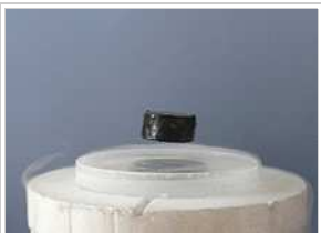
A magnet floating above a superconductor bathed in liquid nitrogen demonstrates perfect diamagnetic levitation via the Meissner effect. Experiments with an ampere-based definition of the kilogram flipped this arrangement upside-down: an electric field accelerated a superconducting test mass supported by fixed magnets.
