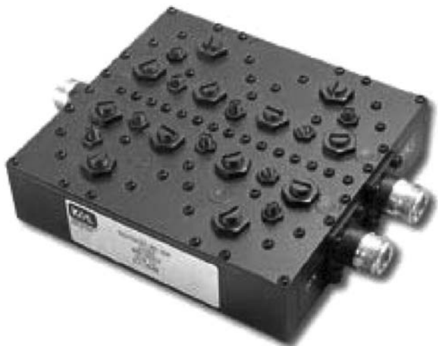
Figure 31. A 1.8-GHz DCS duplexer.
