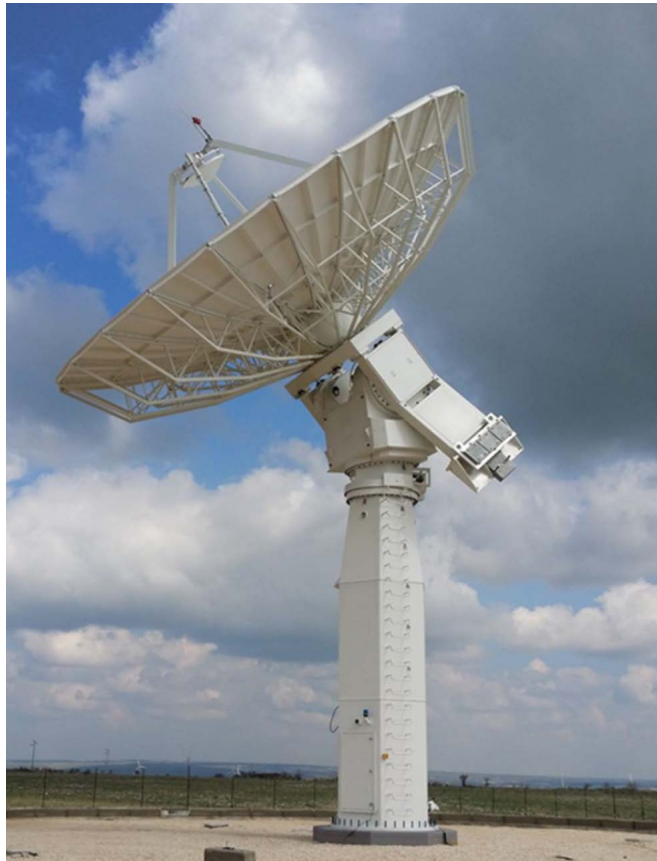
Figure 6.1: X-band ground station with d = 11.28\text{ m}
