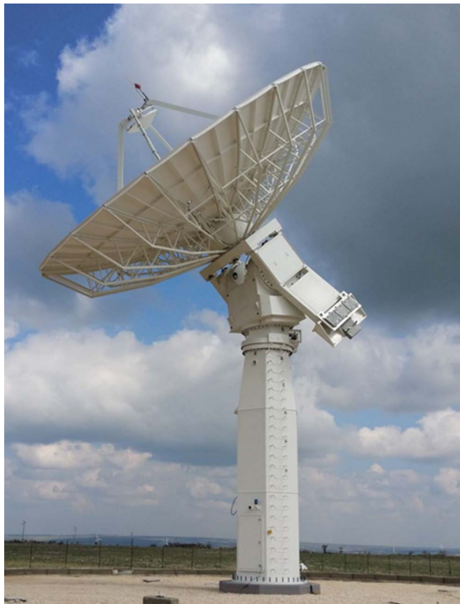
Figure 6.1: X-band ground station with d = 11.28\text{ m}
