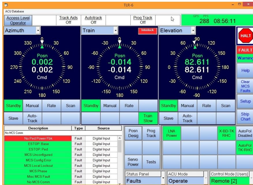
Figure 6.2: Software for antenna remote control
