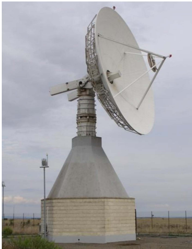
Figure 3.1: Example of X-band ground station antenna with d = 10 m
