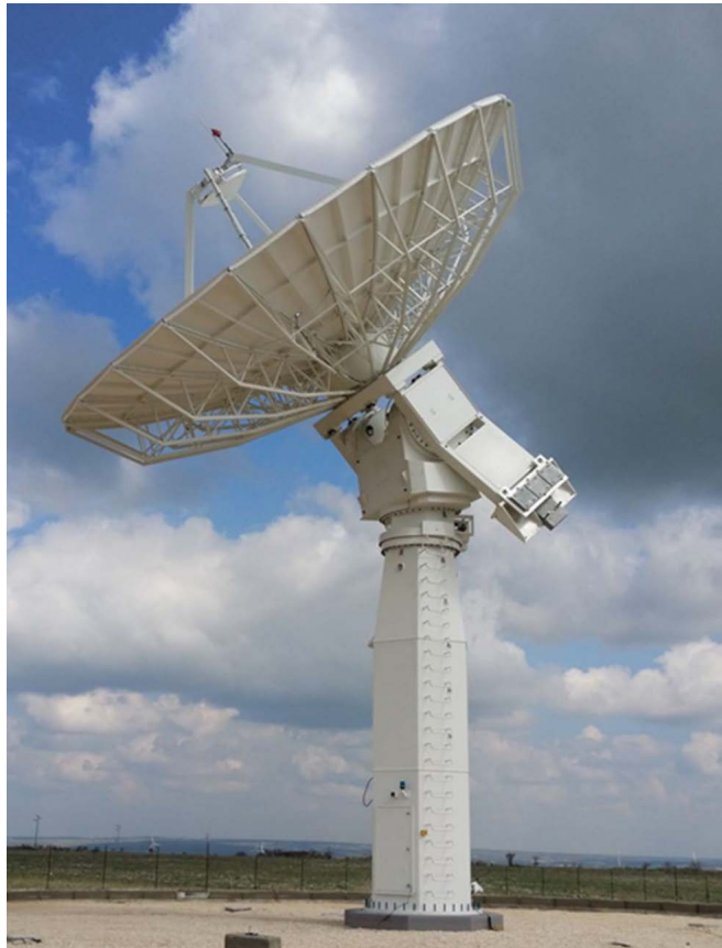
Figure 6.1: X-band ground station with d = 11.28\text{ m}
