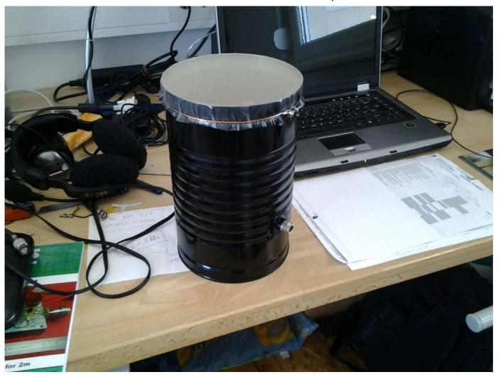
Results are better for 0.3 dB compared to septum feed tuned to  $1300 \ MHz$
