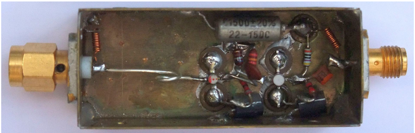
Figure 8: Practical implementation of the LNA.
