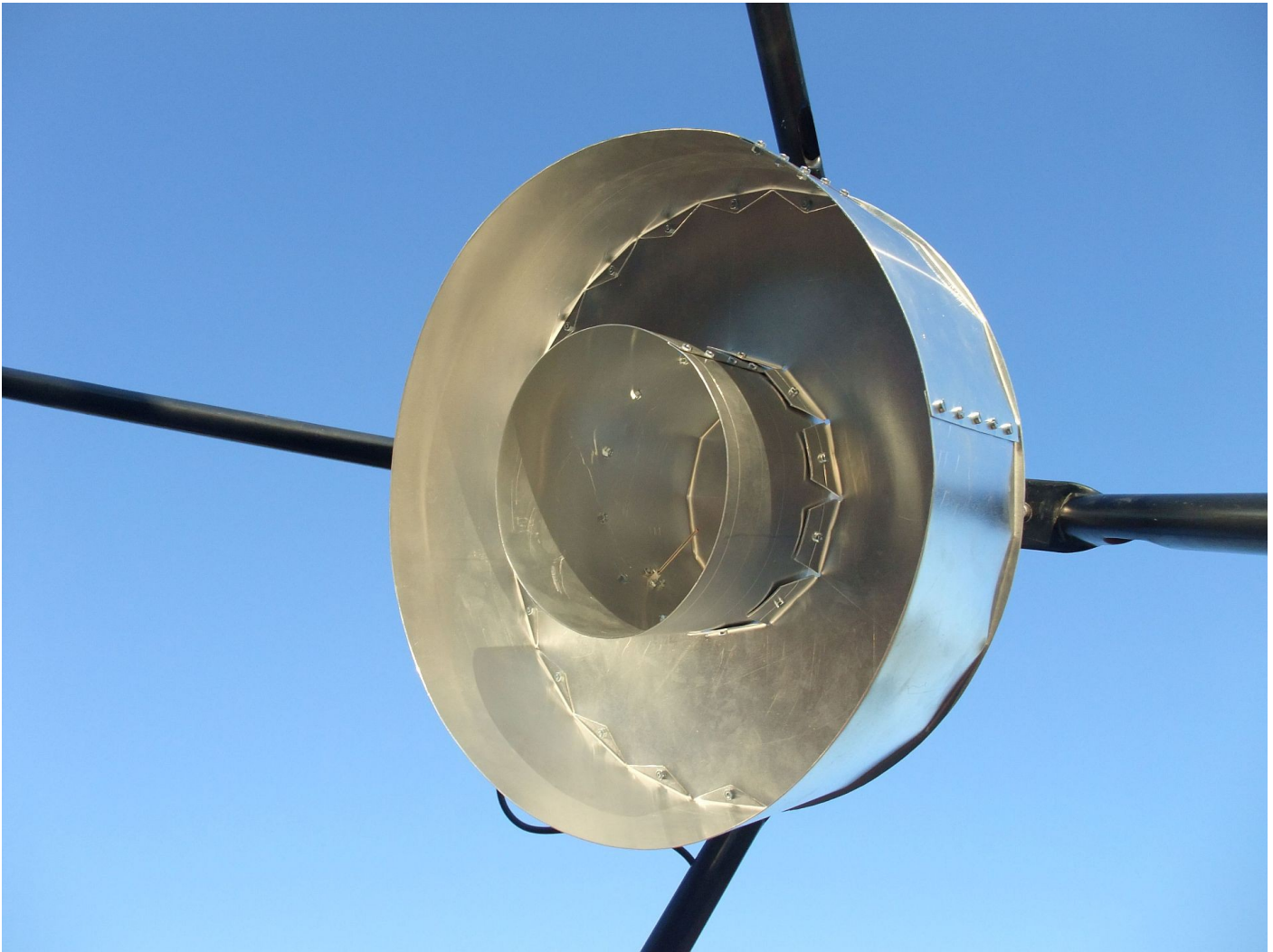
Figure 4: Practical implementation of the VE4MA feed.
