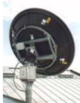
Shown here is a heated 1.5 m parabol antenna from Hirschmann (Technical Museum Vienna/Austria)
