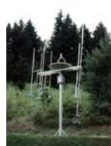
Shown here is a rotor (360° AZ/90° EL) supporting a 90 cm parabolic bowl antenna in the center. A 4.8 m long cross Yagi antenna for the 70 cm UHF-band and a Sat S-band antenna (13 cm/2 GHz) are also positioned by means of a crossbeam of 180 cm length.
