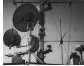
Shown here is a rotor (360° AZ/90° EL) supporting a 90 cm parabolic bowl antenna in the center. A 4.8 m long cross Yagi antenna for the 70 cm UHF-band and a Sat S-band antenna (13 cm/2 GHz) are also positioned by means of a crossbeam of 180 cm length.
