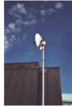
EGIS-Rotor (AZ = 360°; EL = 90°) in duty at the department for "Astronautic and Space Science" at the "Deutsches Museum", Munich. Weather satellites (LEOs) are scanned permanently.
