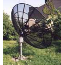
Rotor with 3.1 m mesh-primefocus antenna for C-band reception
