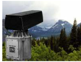
Right here (in the alps) a live weather panorama cam follows the terrain profile controlled in two axis via RS-232-C interface.
