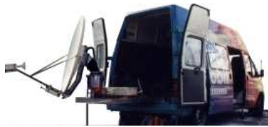
SNG truck of "Antenne Bayern", Munich/Germany in position to uplink news
