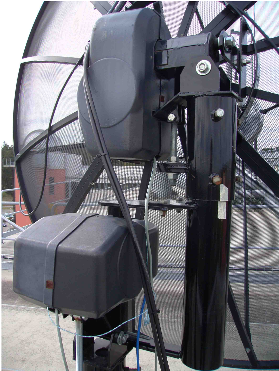
Figure 5.2: The motors, with the bottom one mounted perpendicular to the top motor.
