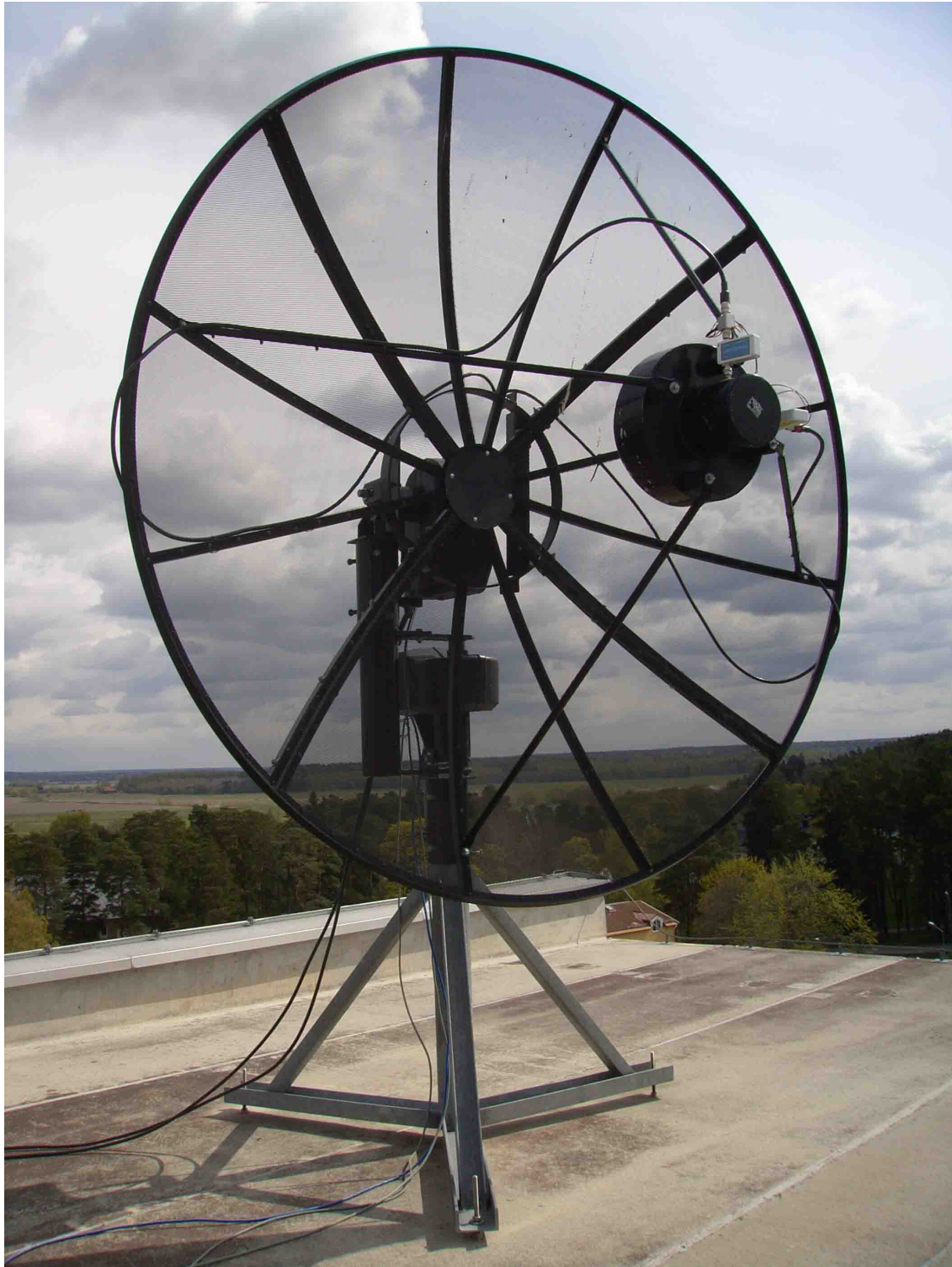
Figure 5.1: The dish in its final stage with all cables and amplifiers connected, pointing at the reset point, Azimuth 270 degrees and elevation 0 degrees.
