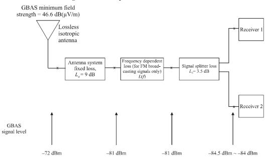
Note 1 – Typical aircraft installation includes a signal splitter to feed two aeronautical receivers. Note 2 – The frequency dependent loss L(f), is equal to 0 for aeronautical frequencies and therefore does not appear in formula (3).
