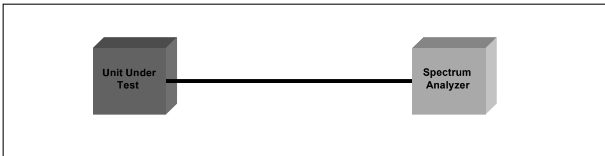
Figure 16-1. Residual Radiation Test Equipment Configuration
