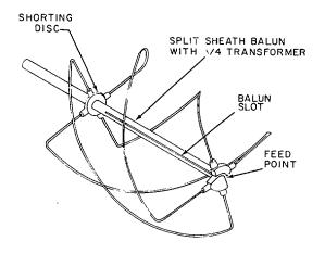
FIGURE I QUADRIFILAR HELIX ANTENNA
