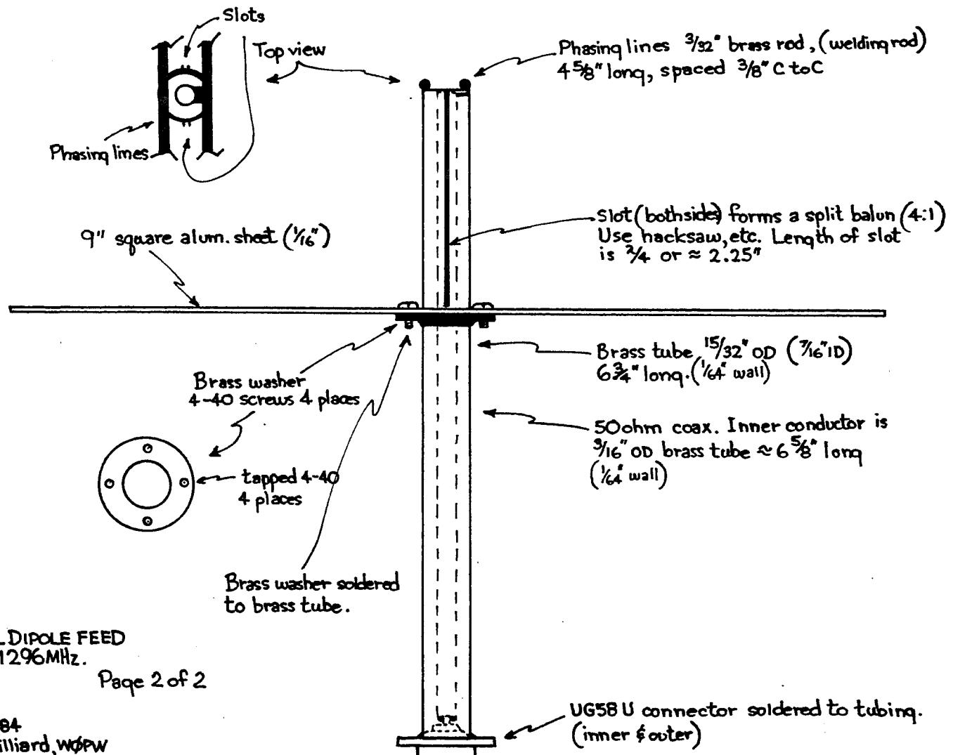
A 32 ELEMENT LOOP YAGI FOR 1296 MHz
