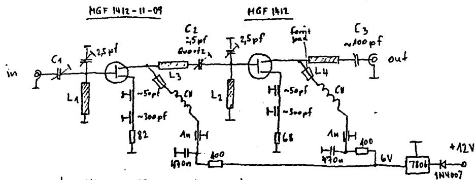
Measurements: NF < 0.6 dB, 2300 MHz, gain 32 dB
