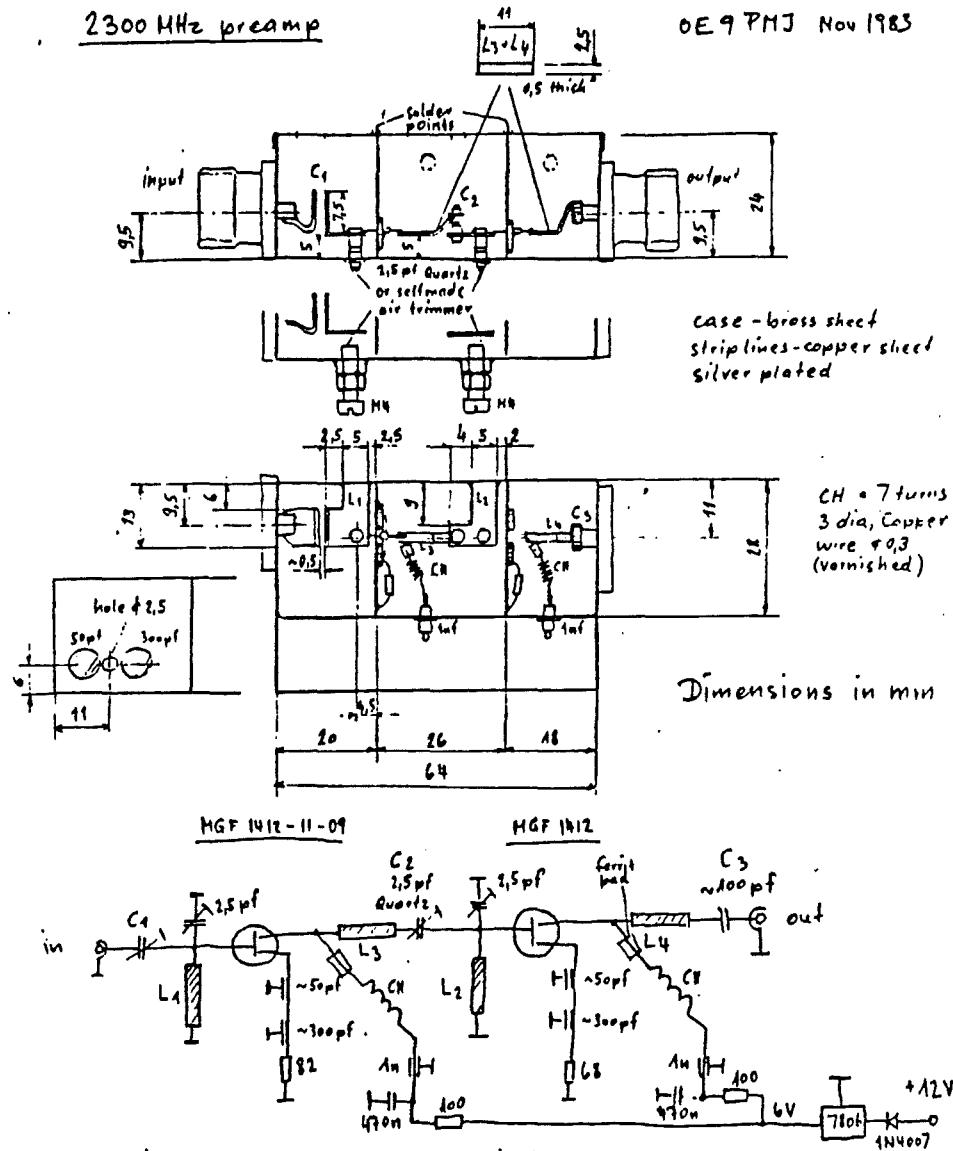
Measurements: NF < 0,6 dB, 2300 MHz, gain 32 dB
