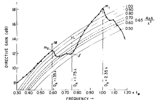
Fig. 2. Directive gain versus frequency curve.
