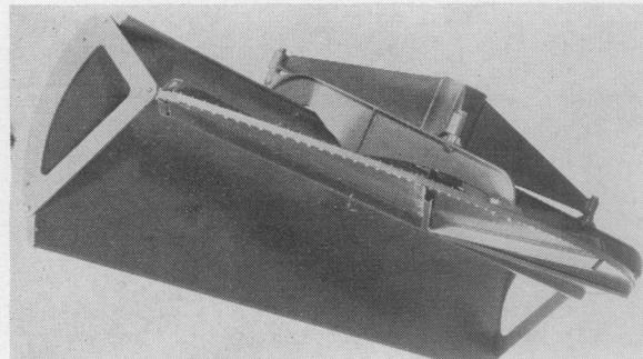
Fig. 4—Pillbox antenna feeding a cylindrical reflector.
