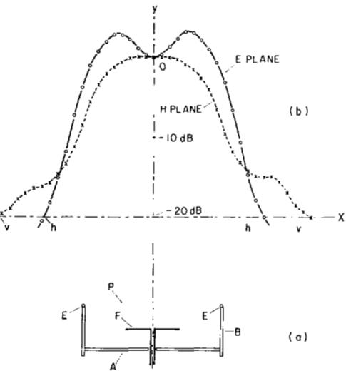
Fig. 5. Amplitude distribution in aperture of antenna.
