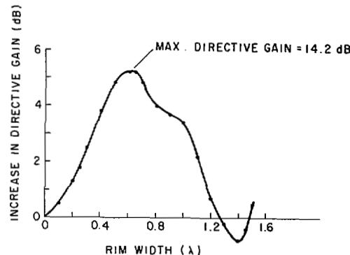
Fig. 3. Effect of rim width on directive gain.
