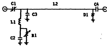
C1 20 or 60 pF variable -- resonates with L2 at input freq.
