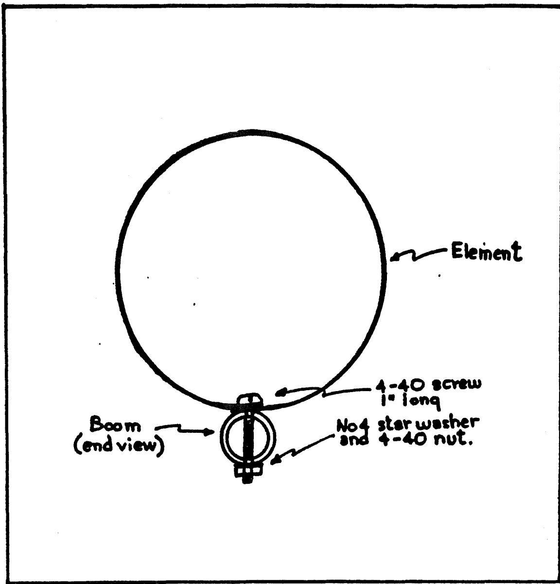
Figure 3 - How the elements are mounted
