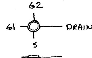
Q1 NE41137 GaAs DUAL GATE MESFET (CALIFORNIA EASTERN LABORATORIES)
