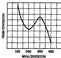
Fig. 12 Harmonic Performance of the Circuit Shown in Figure 4 at 1 dB Gain Compression
