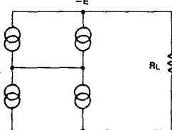
Fig. 9 Adding Two Current Sources to Double the Current
