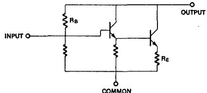
Fig. 1 RB - Shunt Feedback Resistor
