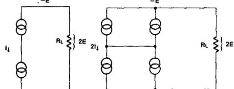
Fig. 8 Electrical Equivalent without Transformer
