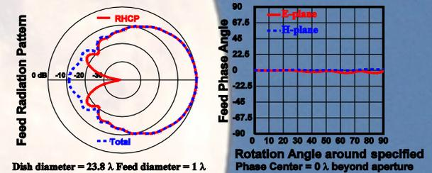
Dish diameter = 23.8 λ Feed diameter = 1 λ
