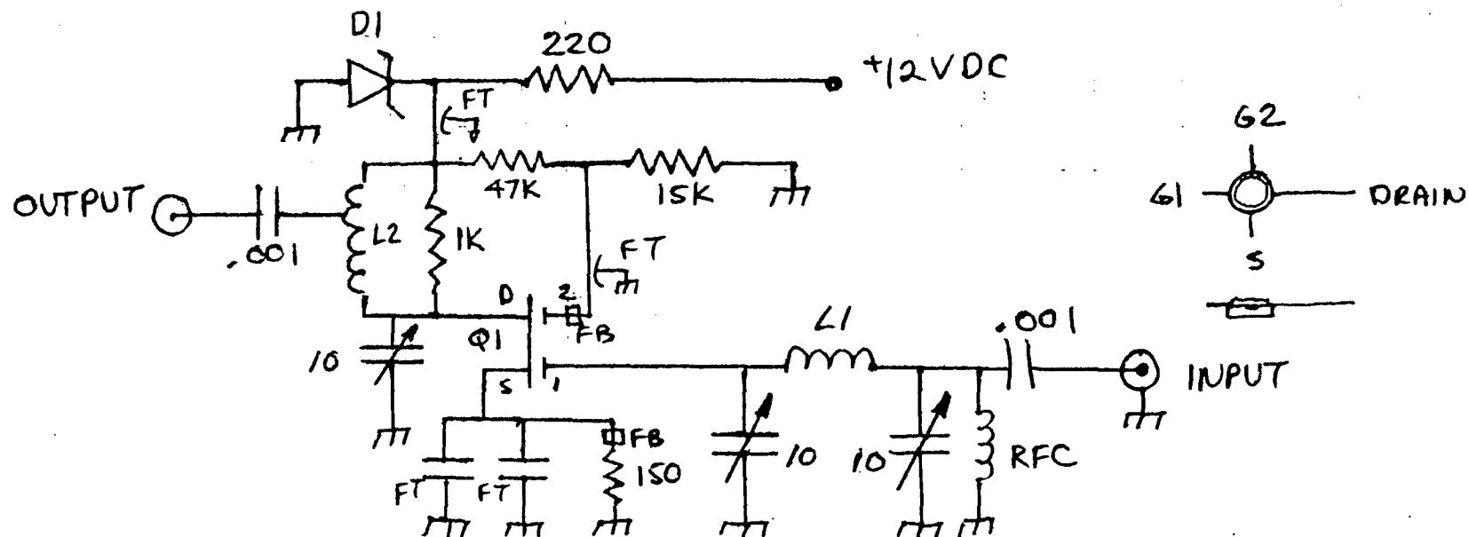
Q1 NE41137 GaAs DUAL GATE MESFET (CALIFORNIA EASTERN LABORATORIES)
