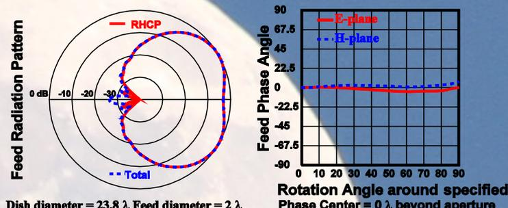
Dish diameter =  $23.8 \lambda$  Feed diameter =  $2 \lambda$
