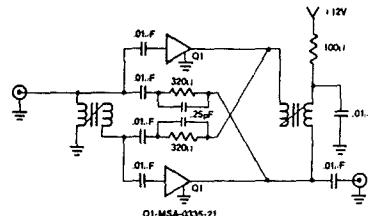
Fig. 11 Unilateraled Push-Pull Circuit
