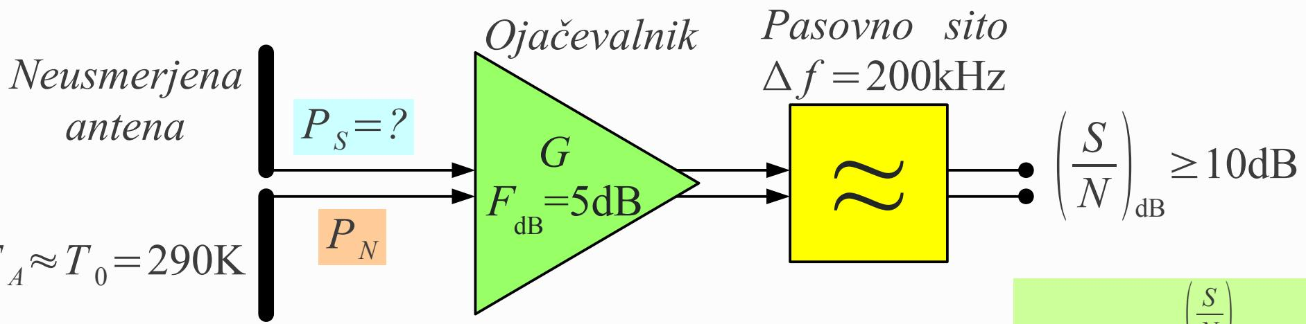
$$T_G = T_0 \cdot \left( 10^{\frac{F_{\text{dB}}}{10}} - 1 \right) = 290\text{K} \cdot (3.162 - 1) = 627\text{K}$$
