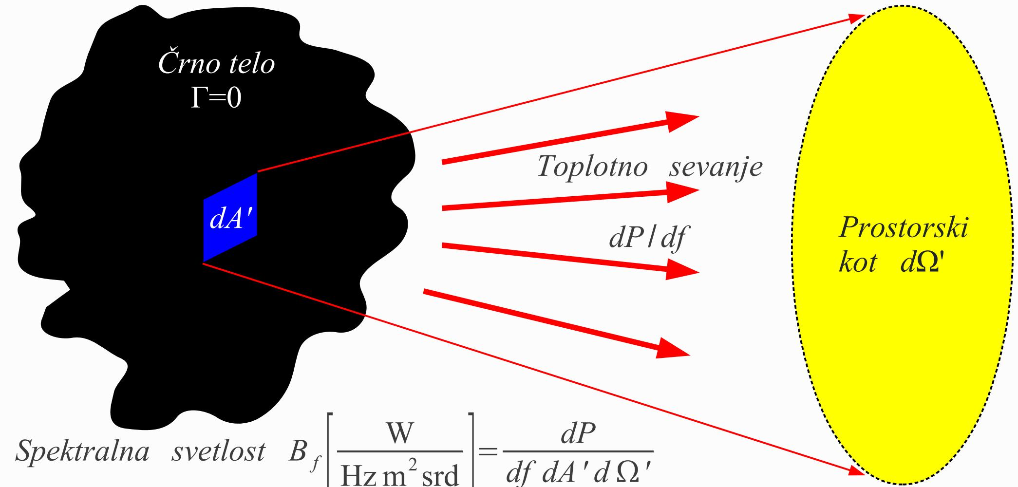
$$B_f \left[ \frac{\text{W}}{\text{Hz m}^2 \text{srd}} \right] = \frac{dP}{df dA' d\Omega'}$$
